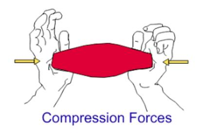
Compression is a pushing force. The application of power or pressure against an object causes it to become squeezed, squashed or compacted.
